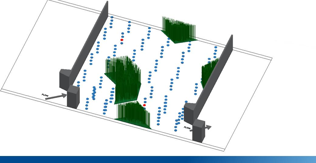
Flow and turbulence structure in a vertical slot—brush fish pass
