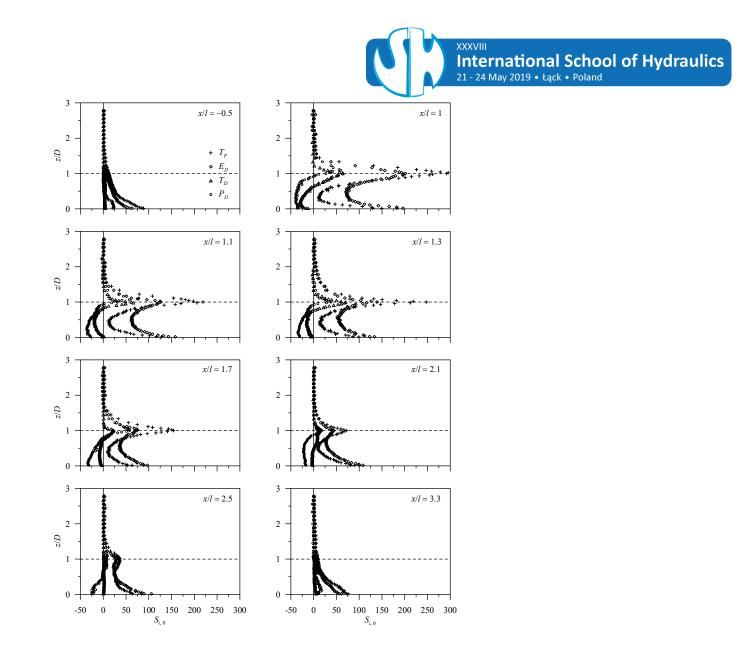
**Fig. 9** TKE budget components  $T_P$ ,  $E_D$ ,  $T_D$  and  $P_D$ , as a function of z/D at different streamwise distances for Run 1.
