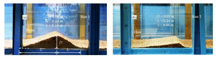
**Fig. 1** Photographs of the dunal structures for (a) Run 1 and (b) Run 2.
