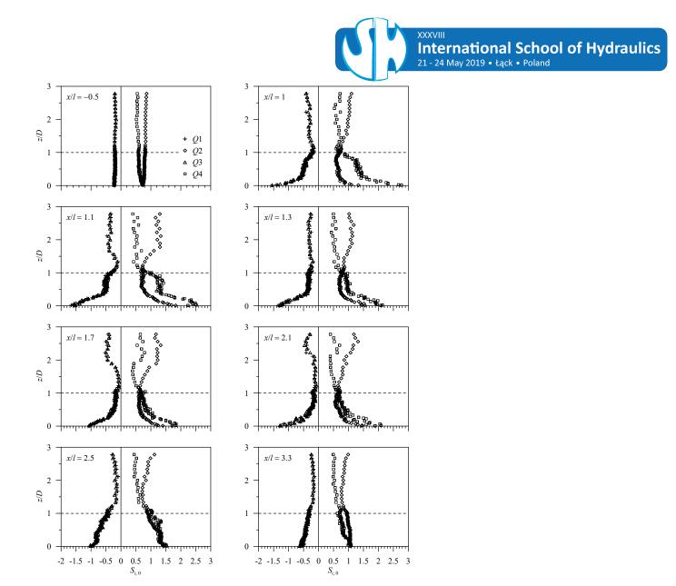
**Fig. 8** Variations of  $S_{i,0}$  with z/D at different streamwise distances for Run 1.
