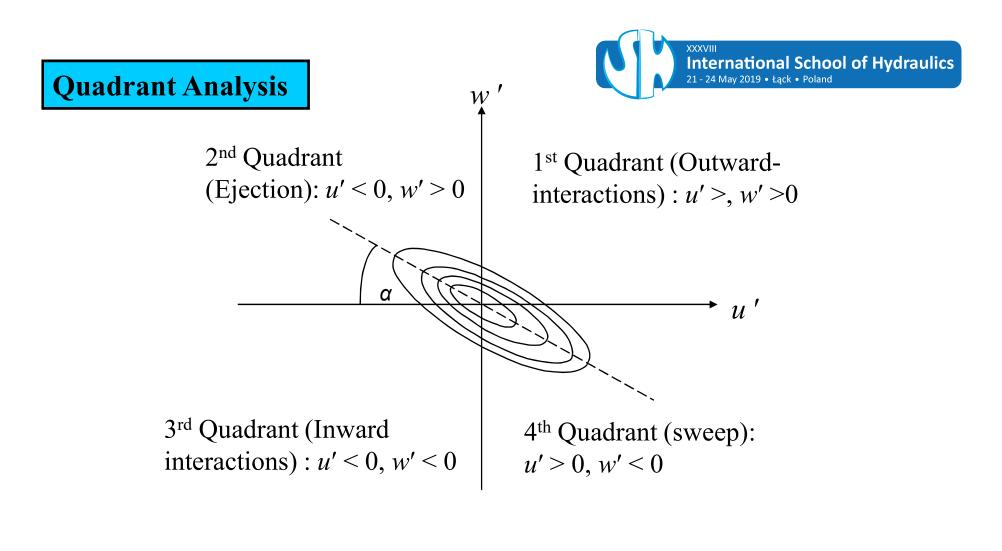
**Fig. 7** Quadrant plots of velocity fluctuations (u', w') on u'w'-plane.
