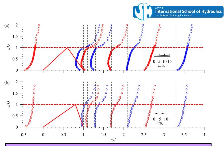
Fig. 3 Vertical profiles of nondimensional streamwise velocity  $u/u_*$  at different streamwise distances for Runs 1 and 2
