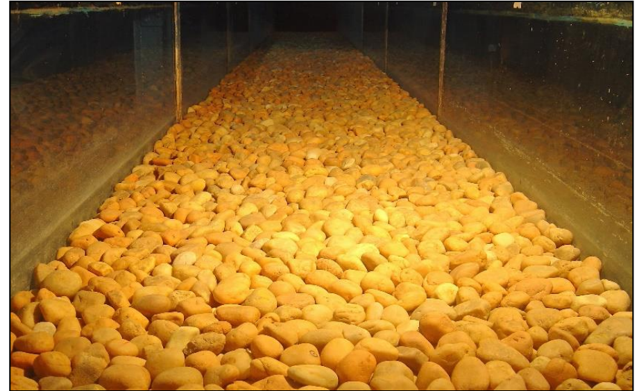
Fig. 3 Photograph of a natural gravel-bed stream (WGB) and a screeded gravel bed (SGB) in a laboratory flume
