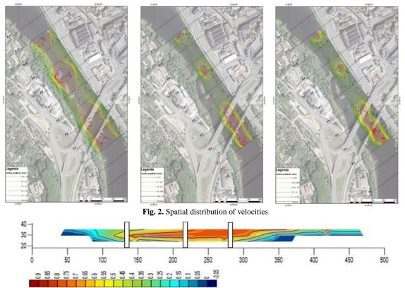
Fig. 3. Magnitudes of the flow velocities in bridge cross section
