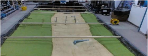
Fig. 1. Physical model with the bridges and elements of the river regulation
