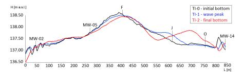
Fig. 1 Longitudinal profiles PR-T along the Kępa Chwałowska Island, Vistula; initial bottom - measured (black), blue and red - calculated bed elevation during and after passage of Wave 2, respectively.
